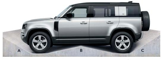
Ride Height Off-road<sup>0</sup> - Coil (Air) Standard - Coil (Air) Approach Angle 31,5° (37,5°)
